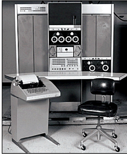
Picture 3: A successor to the PDP-4, the PDP-7 used smaller, more conventional system units and was well received in laboratory and data acquisition applications. The machine featured DEC's first mass-storage based operating system (DECsys for DECtape). Ultimately, 120 PDP-7s were produced and sold. Source: http://www.digital.com/timeline/1964-3.htm .
