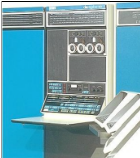
Picture 6: The 36-bit PDP-10 was program-compatible with the PDP-6 and approximately twice as powerful. Designed to perform conversational timesharing, batch-processing and real-time operations equally well and simultaneously, the PDP-10 achieved great popularity with the commercial timesharing utilities, university computer centers and research laboratories. Source: http://www.digital.com/timeline/1967-1.htm .
